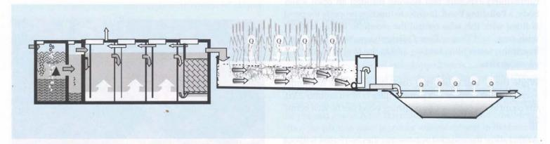
out of the baffled tank reactor and anaerobic filter. If the effluent is reused, a planted filter is added which will take the odour away. With an efficient pretreatment, the size of the planted filter can be reduced to 0.30 m² per person. Granite stones can be used as filter material and even plant species like canans (Cana Indica) are able to grow in planted filters.
