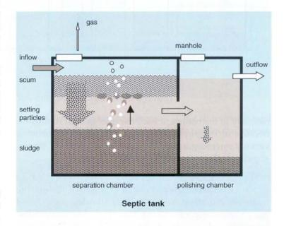
more or less untreated. The treatment efficiency of a septic tank is in the range of 30% COD removal. Desludging at regular intervals is absolutely necessary. A septic tank can also be incorporated into an anaerobic baffled tank as the first section as a **Settler** device.
