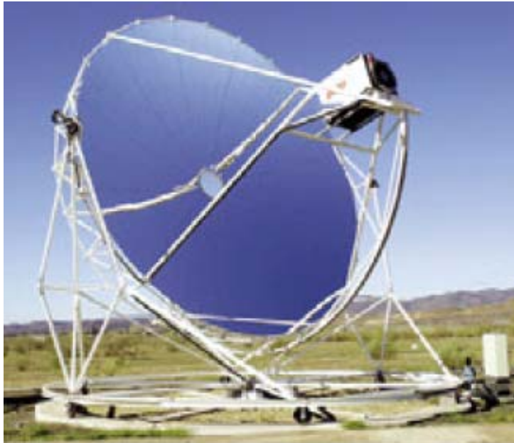
Fig. 33: European project EURODISH, 10 kW Dish engine for decentralized power generation
