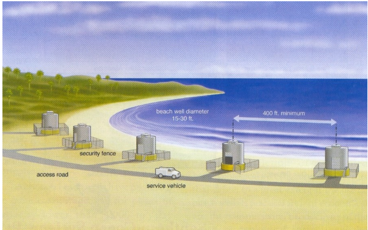
Fig. 55: Sketch of Well Gallery Extraction bore well gallery
