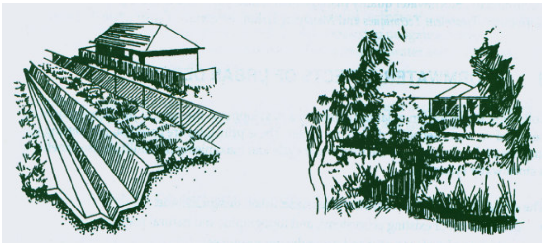
Figure 32 Classical road side drain on the left side and a more natural swale on the right side. The classic type of road side drain is generally considered as not ecological and not to be used in environmentally sustainable towns and cities.
