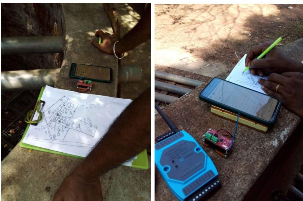
*Azhaganandan (Azha) testing for signal transmitted by water meters*
