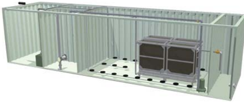
Image 28: MBR system build in pre fabricated containers
