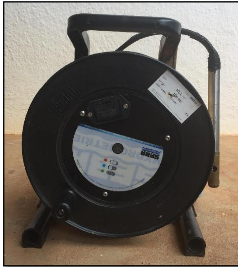
Figure 3—1 Seba Electrical Contact meter used for water level monitoring in wells
