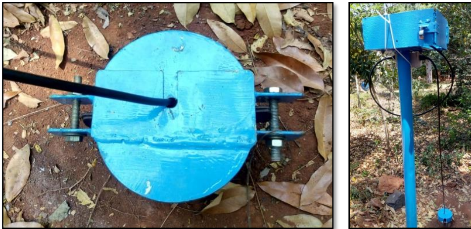
Figure 3—5 Monitoring well metal cover with cable inserted (left), and full set-up of LoRaWAN device (right)
