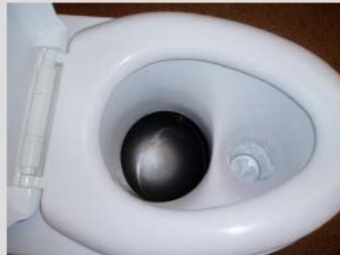
A modern waterless separation toilet has been developed in the China-Sweden Erdos Eco-Town Project (for contact see table 2). The toilet is designed for use in multi-storey buildings and allows dry faeces collection and separate urine collection. Made from ceramics, it has the comfort and aesthetics of a modern flush toilet. It is equipped with a flushing device for ash and a mechanism to seal off the drop shaft.
