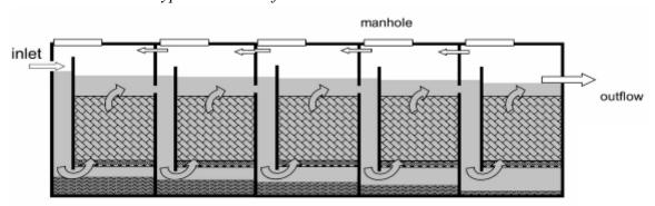
Typical section of an Anaerobic Filter
