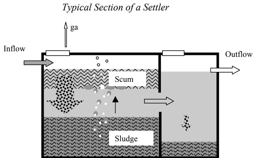
**Desludging** is the process of emptying the sludge at regular intervals from the first and second chamber, which is an absolute necessity. Sludge is composed of helpful bacteria, it is useful to ensure a left over portion in the bottom, in order to provide fresh inoculation material for restarting the process after the regular ( 2 to 2½ year interval) cleaning period.
