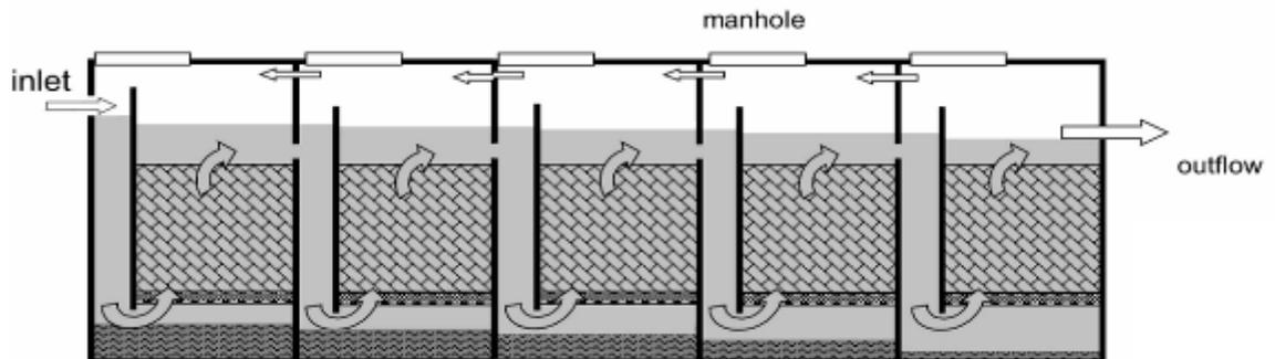
Since the system works in a closed environment without oxygen supply (anaerobic conditions) the effluent will continue to smell despite the fact that a major part of the effluent treatment has occurred already. For this reason an additional treatment is included in the design lay out, being the third treatment in the form of a planted gravel filter.
